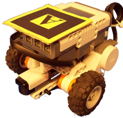
Figure 10: A marker on top of a NXT robot and an infrared sensor is attached in front of the robot.
